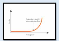
The performance monitor – a light band or needle indicator– shows the level and degree of grain loss and so allows the operator to drive just below point of overload.
