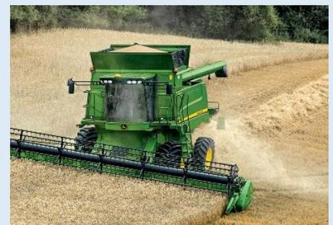
six stepped straw walkers which continue separating the grain from the straw. As there is a limited amount of concave wrap around the threshing drum – up to 120 degrees – there is only a limited time in which threshing can take place. As a result conventional combines need straw walkers to complete the separation.
